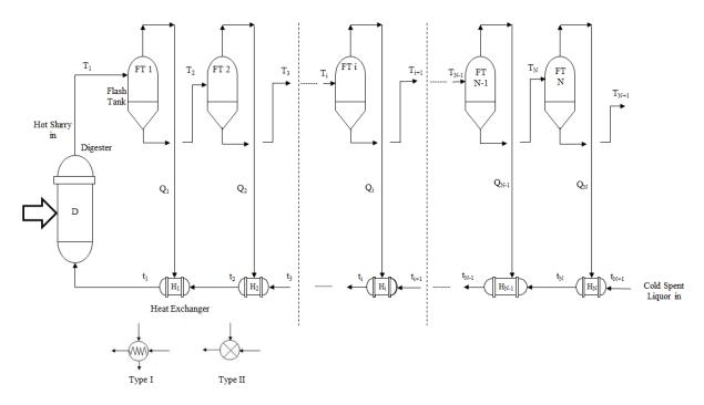
Figure 4: A cascade of the flash tank - condenser units
