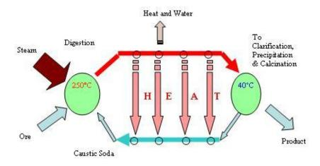
Figure 1: Basic thermal flow chart of the Digester-Precipitator area for the Bayer process.
