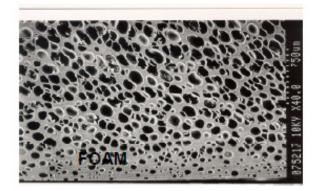
Figure 4: Foam structure: there are comparatively fewer bubbles at the bottom (the cooled surface) than at the top, which is at the half-width.
